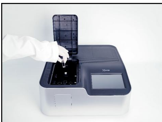
[Figure 1]. Alpha UV-Vis spectrophotometer - A double-beam UV-Vis spectrophotometer developed by K LAB, supporting a wavelength range of 190-1,100 nm and providing stable ultraviolet data required for calculating the K_s and \Delta K values of olive oil.
